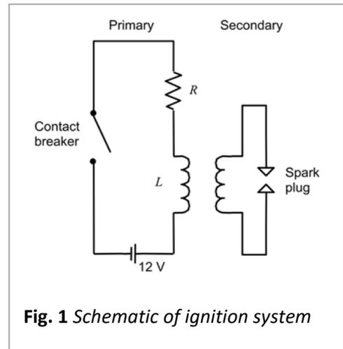
Fig. 1 Schematic of ignition system
