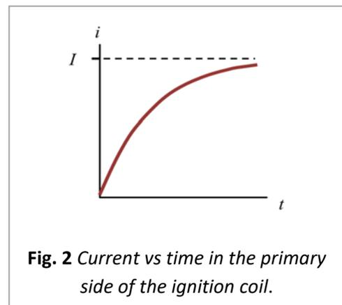
Fig. 2 Current vs time in the primary side of the ignition coil.
