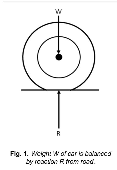
**Fig. 1.** Weight  $W$  of car is balanced by reaction  $R$  from road.
