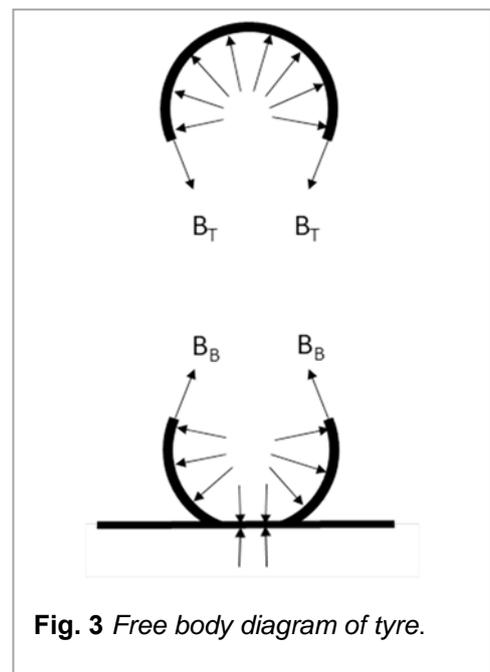
**Fig. 3** Free body diagram of tyre.
