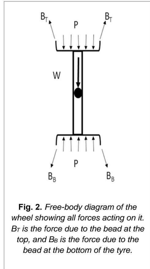
**Fig. 2.** Free-body diagram of the wheel showing all forces acting on it.  $B_T$  is the force due to the bead at the top, and  $B_B$  is the force due to the bead at the bottom of the tyre.
