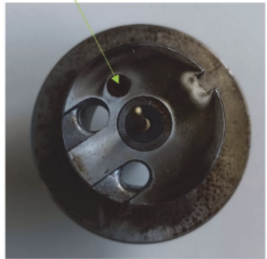
Figure 5 - Underside of Piston showing Piston Cushion
