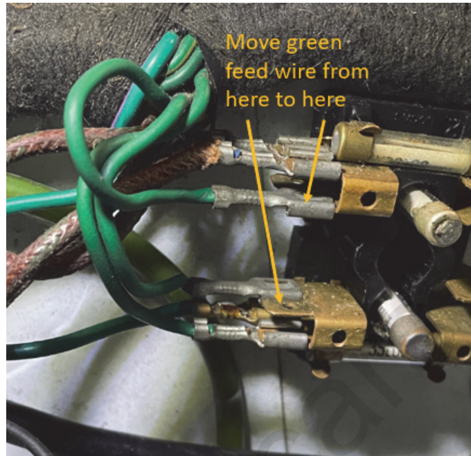
Fig. 10 Flasher relay power moved from fused, switched battery feed to fused battery feed.
