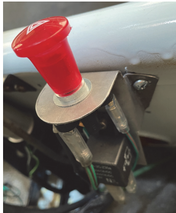
Fig. 4 Parcel shelf switch installation using Switch Bracket.
