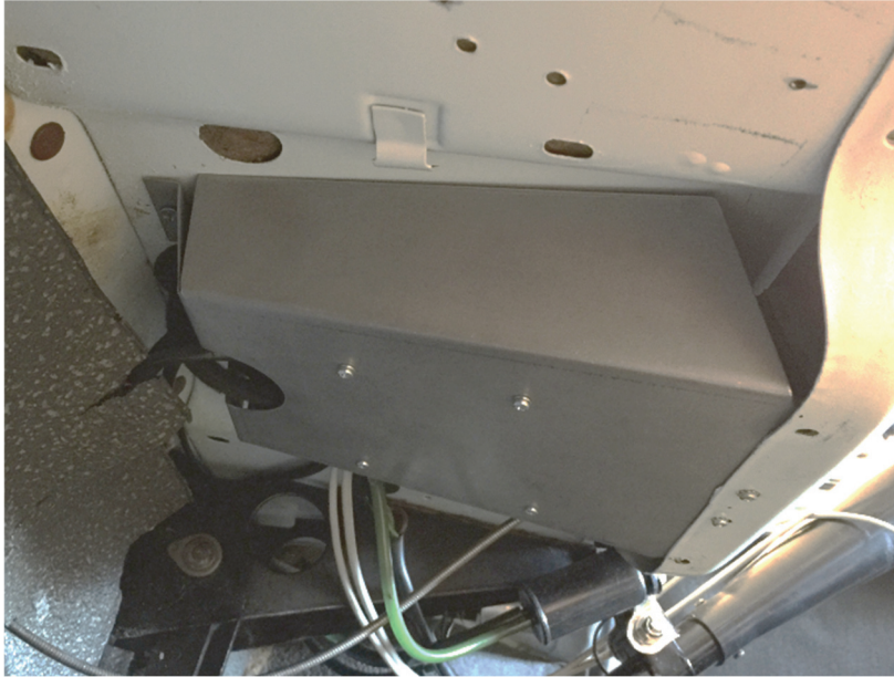
Fig. 3 MINITRON installation under parcel shelf with optional switch shield.
