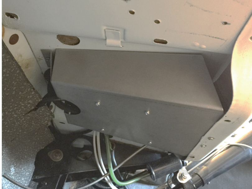
Fig. 2 MINITRON switch shield installation.
